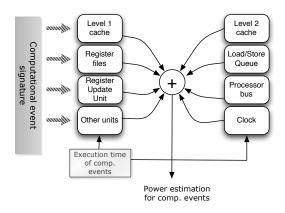
Fig. 4. Different components in the microprocessor power model
