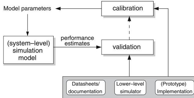
Figure 1. Validation and calibration of architectural simulation models.
