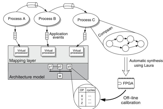
Figure 5. Off-line calibration of dedicated model components.
