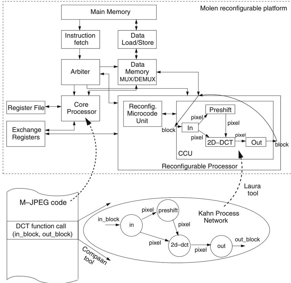
Figure 7. Model calibration for the DCT task using the Compaan/Laura tool-set and the Molen reconfigurable platform.
