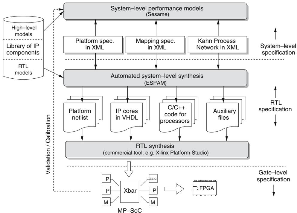
Figure 6. System-level model validation and calibration using the ESPAM design flow.
