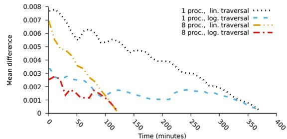
Figure 4: Progression of the *weighted mean* (with respect to the result obtained by exhaustive evaluation) of the execution time distributions for benchmark *bubble sort* (*TACLeBench*).
