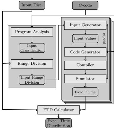
**Figure 2: Toolchain of the EDiFy Framework.** The input to the framework are the C-code, and the Input distributions for each input variable, the output is the corresponding execution time distribution. The left part of the toolchain (input preparation) is executed exactly once, whereas the right part (measurements) is executed iteratively and distributively.
