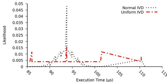
**Figure 6: Execution time distribution for benchmark *ptrch* (EEMBC)**
