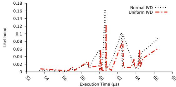
**Figure 5: Execution time distribution for benchmark *bitmnp* (EEMBC)**
