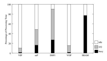
Figure 7: Simulation results showing the utilization of architecture components in *P*1. The throughput is 154.2 frames/sec.
