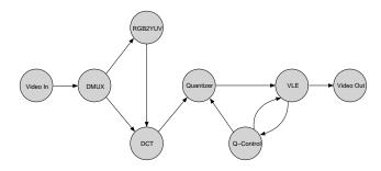
Figure 4: M-JPEG\* encoder application model.
