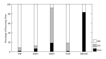
Figure 8: Simulation results showing the utilization of architecture components in P2. The throughput is 82.9 frames/sec.
