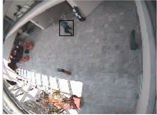
Figure 6: Selection window defines the object region, and it is expanded on each side by 30 pixels to form the background region
