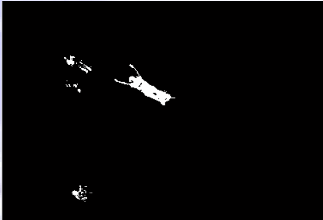
Dilated image multiplied by the subtracted image to get rid of all noise and still keep object contour
