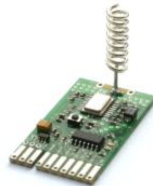
Fig. 1. Wireless network node to which sensors can be attached.
