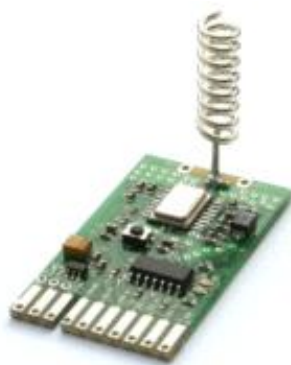
Figure 1. Wireless sensor node used: RFM DM 1810.
