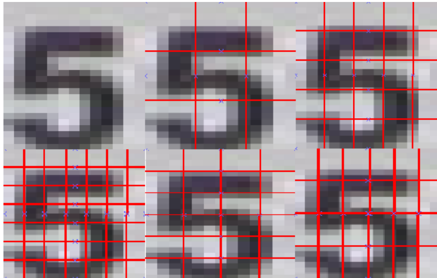
FIGURE 4.11: Grid combinations (top) original image, 3x3 grid, 5x5 grid, (bottom) 7x7 grid, 6x4 grid, 4x6 grid
