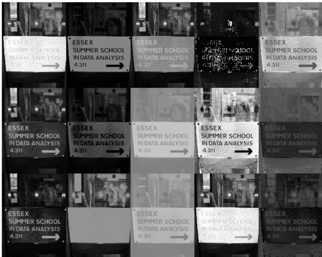
FIGURE 2.1: All color channels 1st column: RGB, 2nd column: O1, O2, O3, 3rd column: Lab, 4th column: HSV, 5th column: rgb
