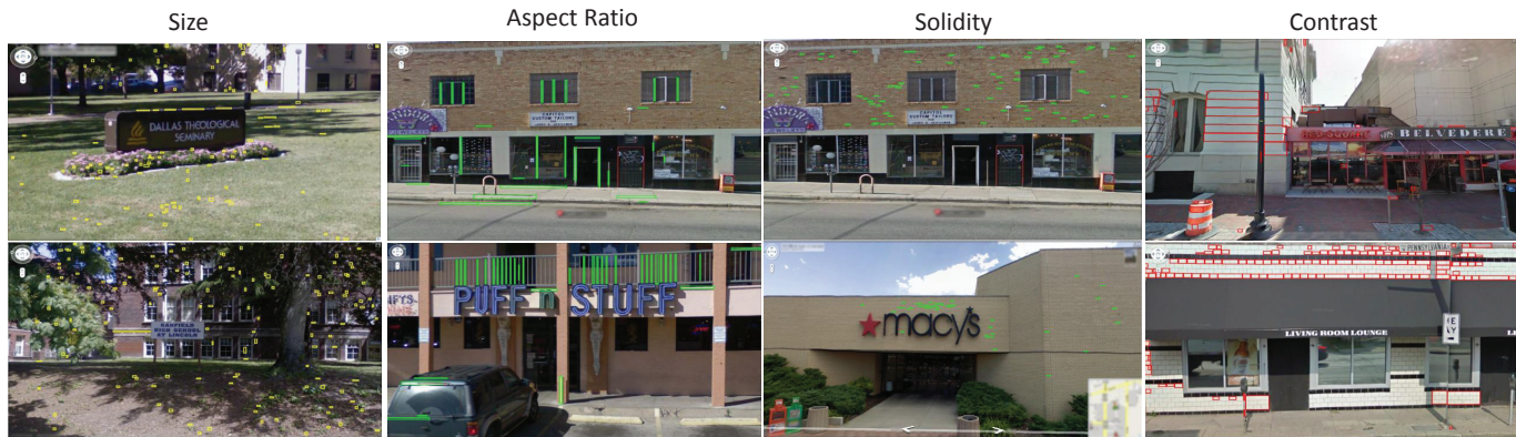
Fig. 5: Samples for character candidate filtering. The green, red and yellow (colors are used to highlight boxes) boxes represent filtered character candidates after corresponding filtering condition is applied (i.e. size, aspect ratio, solidity and contrast).
