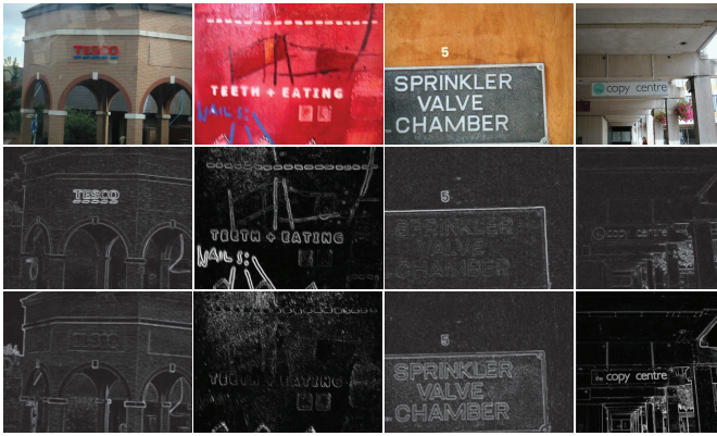
Fig. 3: Saliency map samples: Original images, color saliency and curvature saliency (top to down order). It is shown that text edges are detected better with color saliency for the first two images whereas curvature saliency works better for the last two images.
