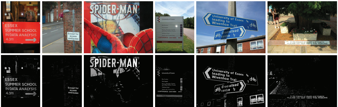
Fig. 6. Original images and text saliency maps obtained. Most of the background regions are filtered out while text regions are preserved by the proposed method. The proposed method is robust against photometric changes e.g., shadow and highlights, text size, style and orientation.
