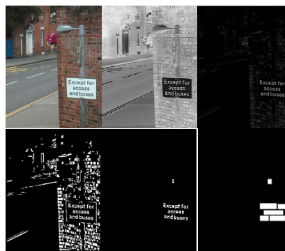
Figure 2. a. Original Input image, b. Inverted Graylevel image of "a", c. Morphological reconstructed image of "b", d. Binarization output of image "c" with proposed method, e. Machine learning process output of image "d", f. Merging output of letters which are extracted in image "e".
