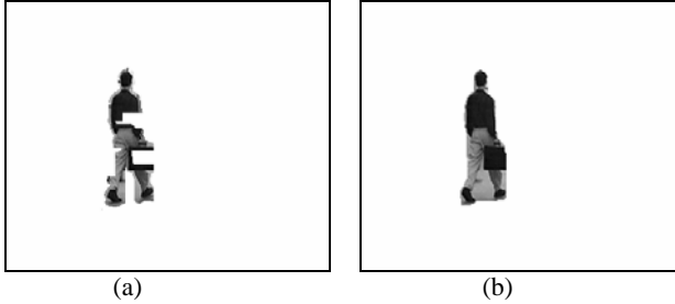
Figure 8. Comparison of results from frame 46 in the “hall” video sequence. (a) The extracted object before the voting process; (b) The result after using the proposed reconstruction approach.
