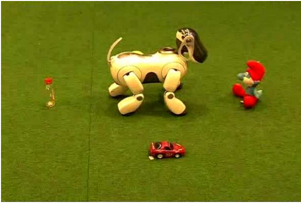
Figure 2. In the recognition phase of our demonstration, the dog will make a 360 degrees turn, recognizing the objects it has learned previously (see also: www.science.uva.nl/~ffseins/aibo.html ).
