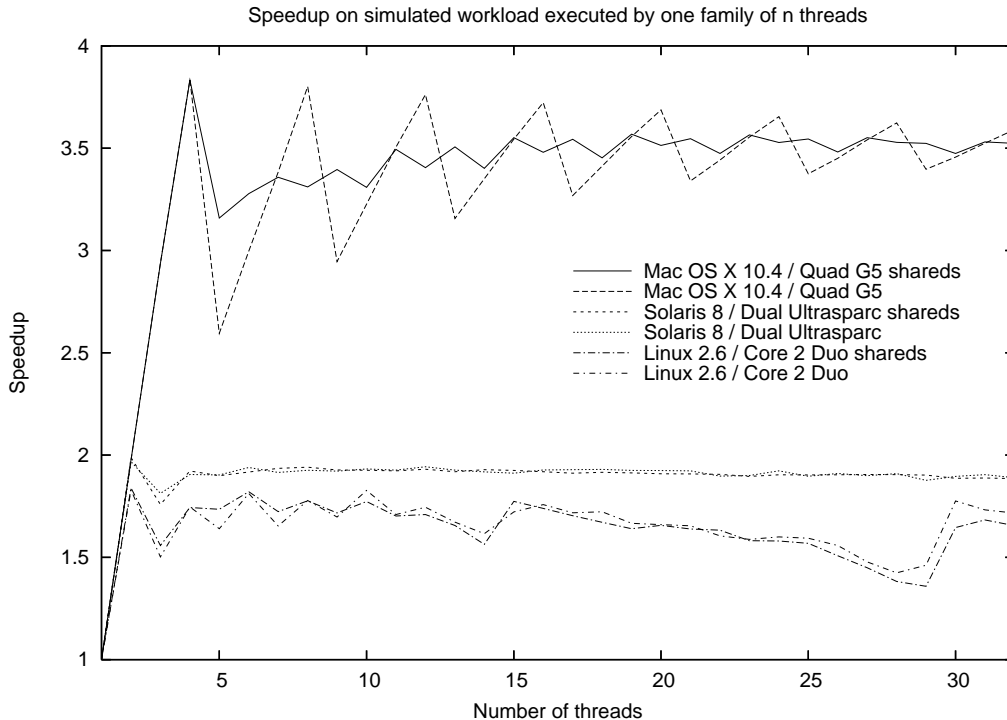
Figure 4. Speedup on simulated workload executed by one family of n threads on several platforms and architectures, with and without the use of shared variables
