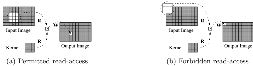
Figure 7: Sequential generalized convolution. Does not represent a parallelizable pattern, as read accesses outside the domain of the input image are possible (see (b)).
