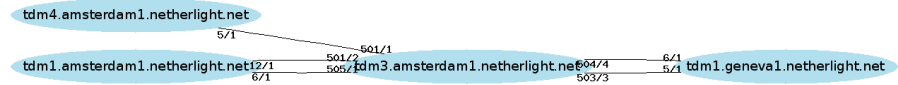
Figure 5.5: A graph of NetherLight resources, as extracted from a NDL file (Source: Van der Ham [p15])
