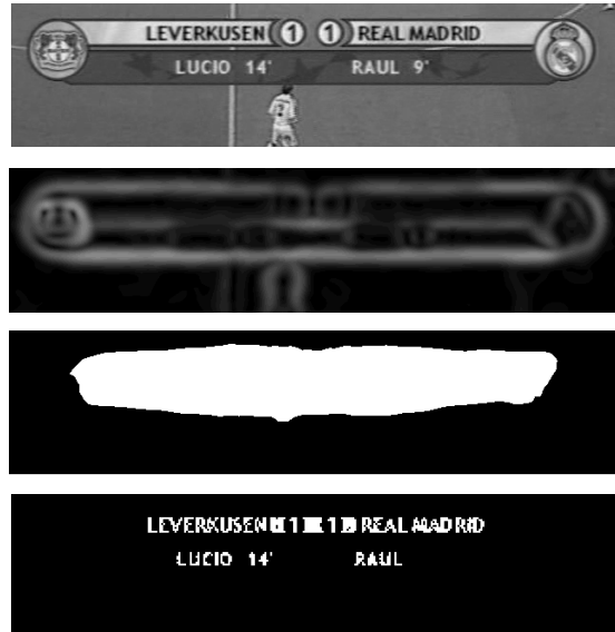
Figure 4: Different steps in overlay segmentation: color edge detection, marked watershed, and Video OCR.
