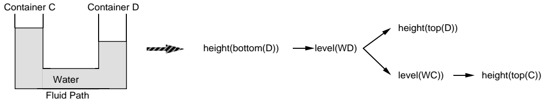
Figure 2.10: Quantity space for the heights in the U-tube
