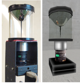
Figure 1: The catadioptric omnidirectional camera, real and simulated.
