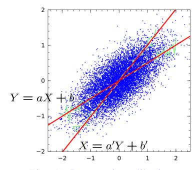
Fig. X Regression dilution regression lines for Y = aX + b + e and X = a'Y + b' + e
