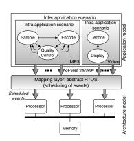
Figure 1: High level scenario-based MPSoC simulation
