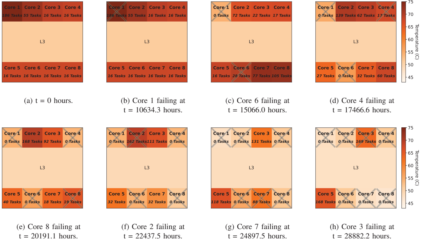
Fig. 7: Heat-map of a CFR multi-core surviving multiple core failures. "X" denotes a failed core. Note that this shows only a single instance of the Monte Carlo simulation and therefore the failing time is a stochastic TTF value and not the MTTF.
