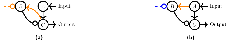
Figure 4: The two reaction networks that can achieve perfect adaptation [17]. (a) NFBN network, and (b) IFFLP network. Orange edges represent saturated reactions, blue edges represent linear reactions, and black edges are unconstrained reactions. Arrowheads represent positive influence and edges ending with a circle represent negative influence.
